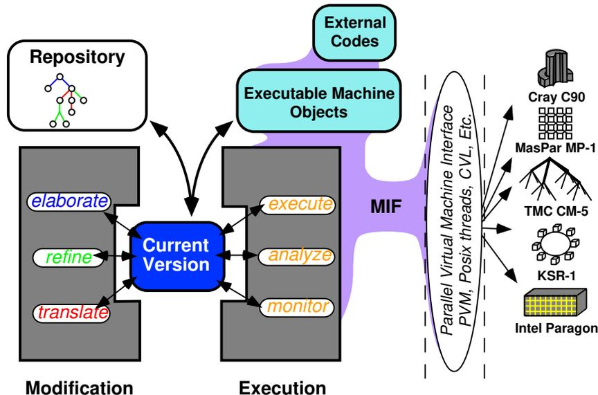
FIGURE 1. The components of the Proteus System
