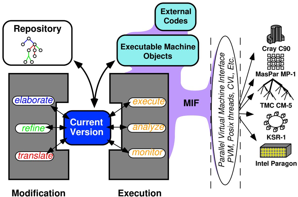
Figure 34 The components of the Proteus System
