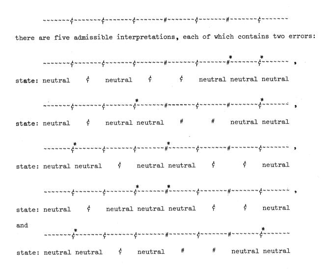
Rather than having all incorrect transitions weigh equally heavily, different "error values" have been assigned to the various types of incorrect transitions, based upon estimates of the likelihood of these transitions.
