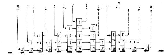
A formatter-symbol which cannot be classified as opening or closing brace and which matches some cell of the stack, is treated as a closing brace; moreover, if it does not match the top, it is treated also as an opening brace. However, in that case, it may not be disregarded in the treatment as a closing brace, since that would give in fact the same interpretation as that in which it is eventually deleted as an opening brace.
