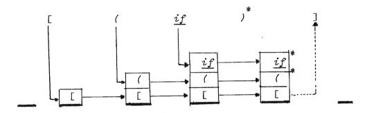
Therefore, in such a case, it will be required that at least one of the opening braces on top of the matching one will be matched away later on, i.e., a transition deleting the last of these braces, if none has been matched away yet, will not be admitted. Note that the requirement that the top cell is matched away whenever possible, is a special case of this general requirement.
