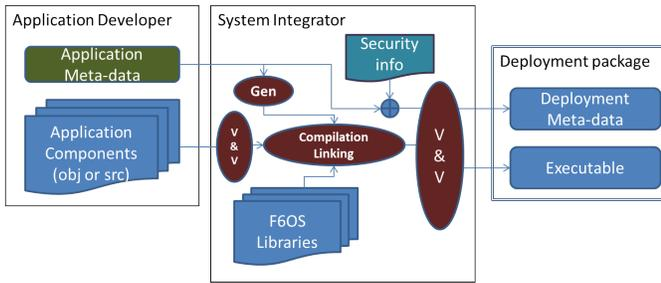
**Figure 11.** Application development and system integration for F6MDA
