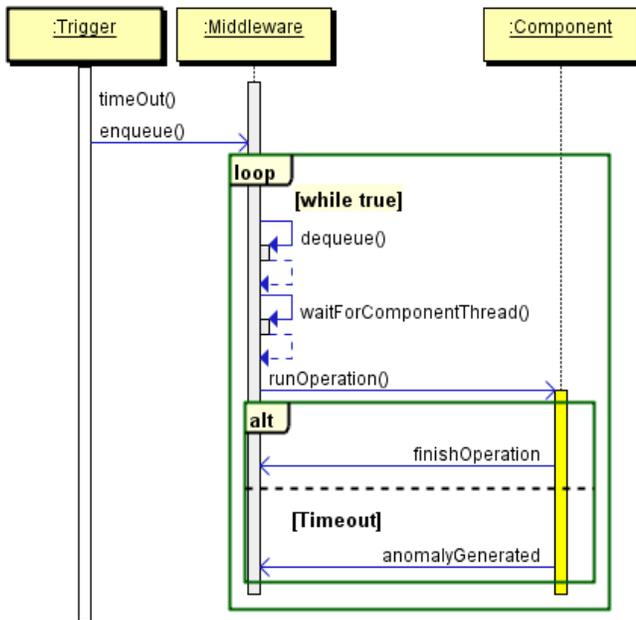
**Figure 6.** Interaction of a time trigger and component
